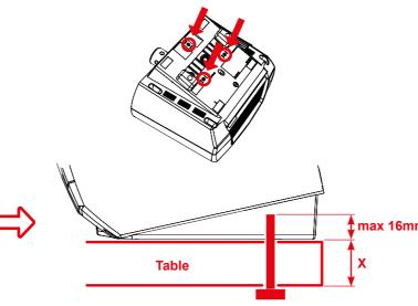
**NOTE:** To hard-mount the CSL Elite Wheel Base + to a table or rig with bolts please, find the printable drilling template in the download area of our website www.fanatec.com
