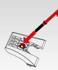
Slide the CSL Elite Wheel Base (A) onto the table top until the limiter blocks stop sliding at the edge of the table.
